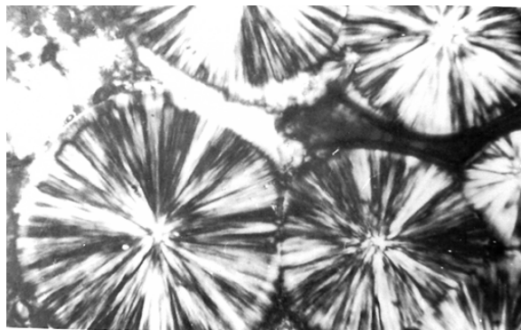
Figure 4.5 An optical micrograph of PP Spherulites
