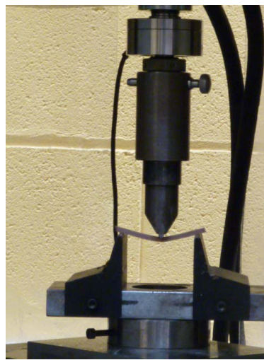
Figure 6.14 A specimen tested in 3-point bending
