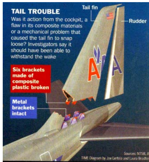
Figure 6.23 Illustration of the aircraft tail section failure at the November 2001 crash (source: TIME, November 26, 2001)
