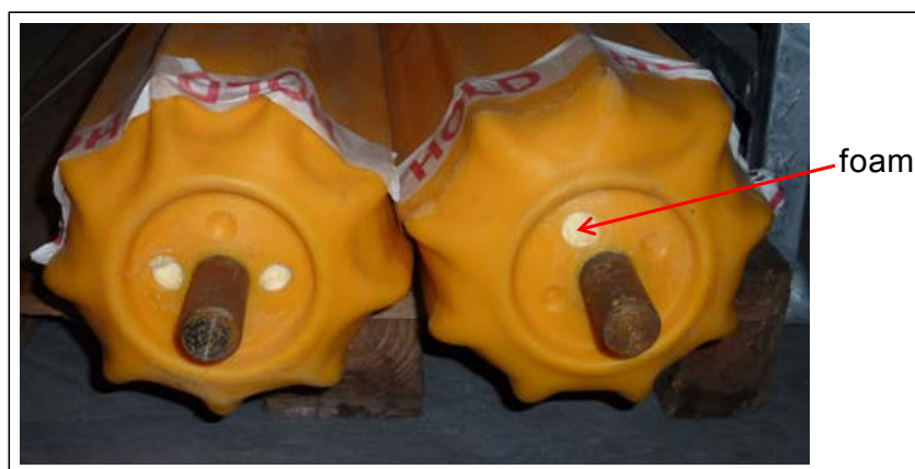
Figure 3.55 Rigid-PU foam filled agricultural rollers (courtesy of JFC Manufacturing Ltd.)
